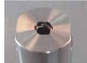
Orifice worn out by slurry
