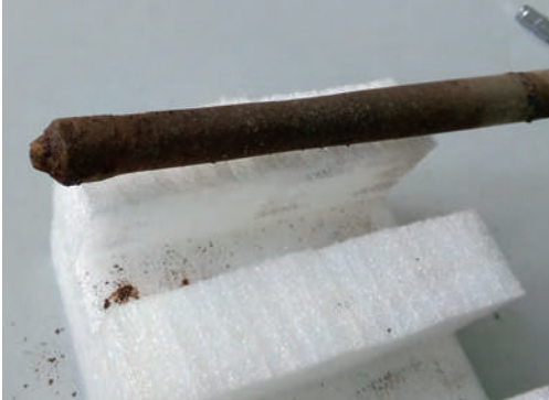
Figure 1 - Heat damage on a stainless steel injection lance
