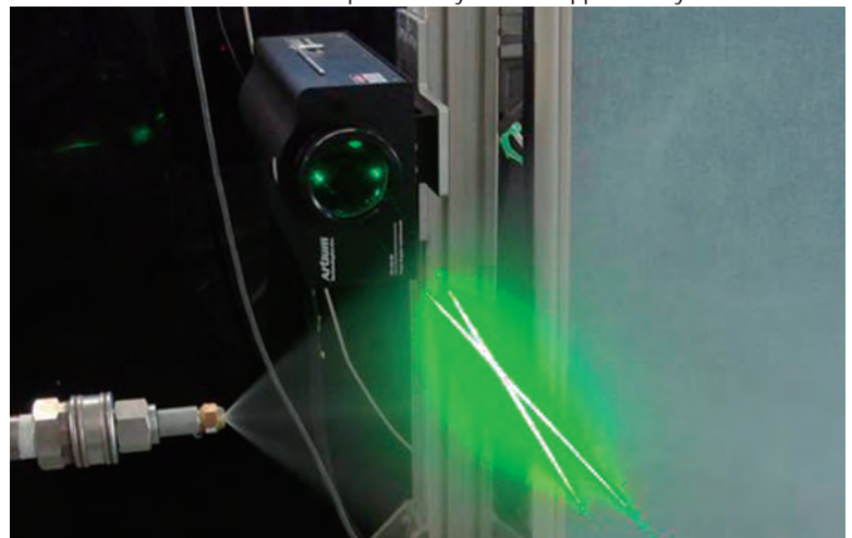
Measurement of droplet size by Laser Doppler analyzer
